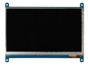
The 7 inch TFT display expands the Raspberry Pi or the Banana Pi with a touchscreen display in no time. It can also be used on any desktop computer and convinces with its high contrast and color-fast display. With a maximum resolution of 1024 x 600 pixels, this display is suitable for any application.
