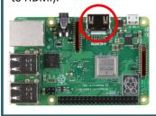
When a Raspberry Pi 4B is used, the HDMI-cable, which features one smaller end is needed (HDMI to Micro-HDMI).
