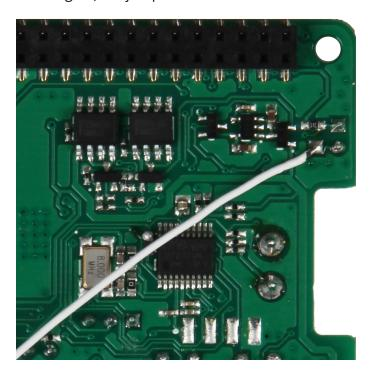
Solder the other end of the cable as shown in the picture below one of the  $\ensuremath{\mathsf{GPIO}}$  pins.
