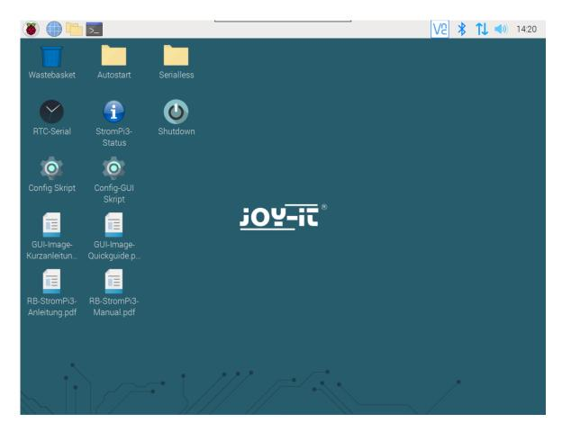
With a double click on **Shutdown**, both the Raspberry Pi and the StromPi will be shut down. Please note that a restart after this is only possible with the help of the PowerOn button modification, a set wakeup alarm, or by removing and reconnecting the power supply.
