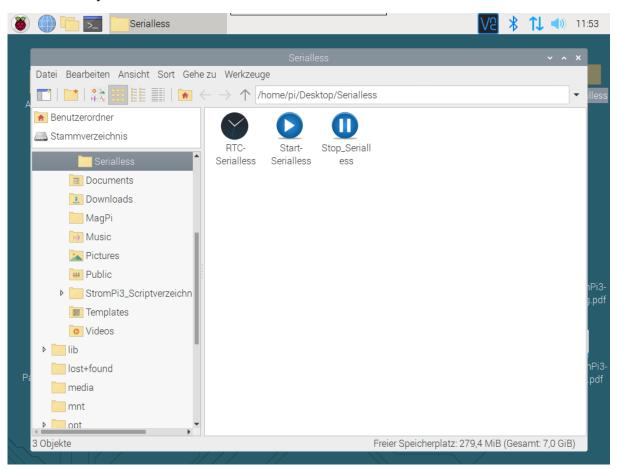
With a double click on **RTC-Serialless**, the time of the Raspberry Pis is compared with the real-time clock of the StromPis and the older of the two times is overwritten with the newer one.
