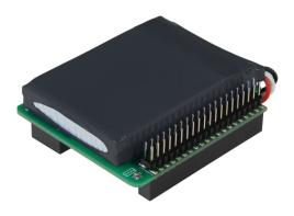
This battery hat turns the StromPi V3 into a full-featured UPS solution. The replacement battery is provided as third current source, is surveilled and will be recharged automatically.
