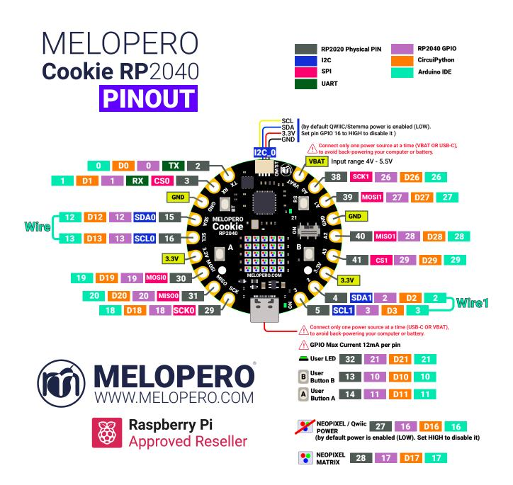
The pinout chart above is useful to quickly find the right name of a specific pin, depending on the language and IDE. As example, note how the pins labeled as 28 and 29 change name depending on which platform you are using to program the board:
