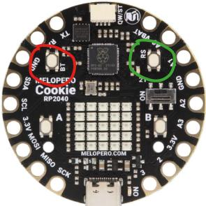
Drag and drop (or copy and paste) melopero\_cookie\_rp2040\_circuitpython.uf2 file to RPI-RP2. The RPI-RP2 drive will disappear and after a few seconds a new disk drive called CIRCUITPY will appear.
